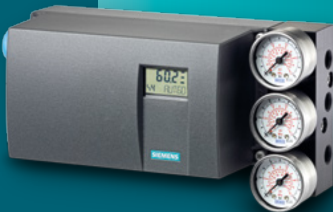
SIPART PS2 – State-of-the-art positioners with innovative features such as non-contact position detection, booster options and extended diagnostics
